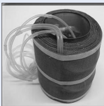
Hand-made twin coil dialyzer
